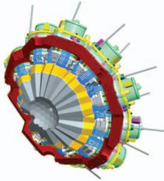
Figure 6.3: The AGATA gamma-ray spectrometer.
