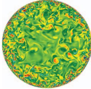
*Figure 9.1: TCross-stream cut of turbulent pipe flow at high Reynolds number, showing colours of axial vorticity. The data was obtained from a high-resolution direct numerical simulation (DNS) using about 25 billion grid points. The fine scales close to the walls and the sharp gradients in the pipe centre are clearly visible which highlights the importance of adequate numerical methods and efficient codes. Image: Philipp Schlatter and George El Khoury.*
